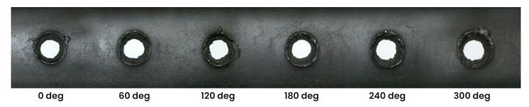
TrueJet perforating charges create uniform entry hole sizes with less than 10% deviation, helping to improve flow efficiency and reservoir access.
