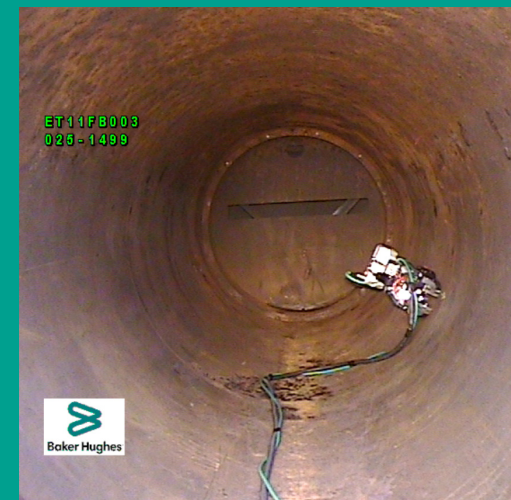
3D-structured light for detailed mapping inside a vessel.
