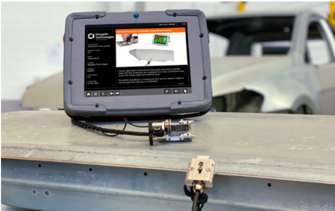
Krautkrämer Bond Scanner allows for the fastest and easiest testing of adhesively bonded parts
