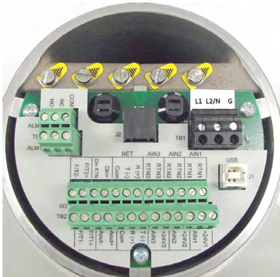
Figure 13: Typical terminal board (three 4-20mA inputs option)
