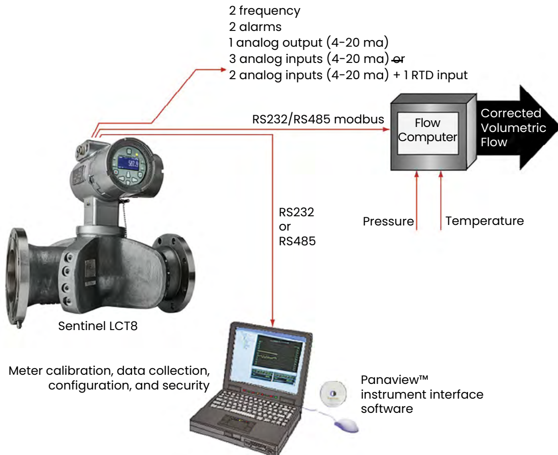
Figure 12: Sentinel LCT8 flow measurement system connections
