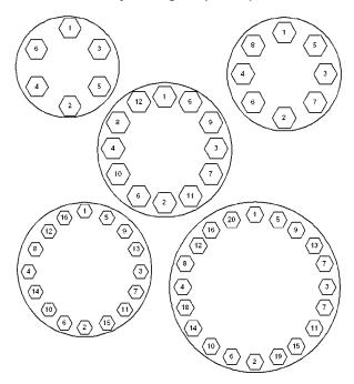
Figure 3: Bolt Torque Sequence
