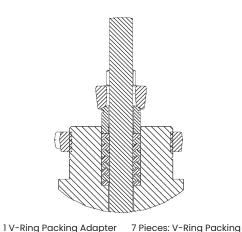
Figure 4: Standard Packing
