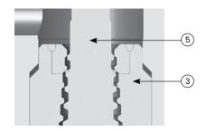
Figure 1: Plug and Seat Surfaces
