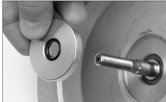
Figure 32 - Installing lower diaphragm retainer
