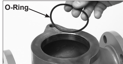
Figure 7a - Remove cage, seat, and o-ring
