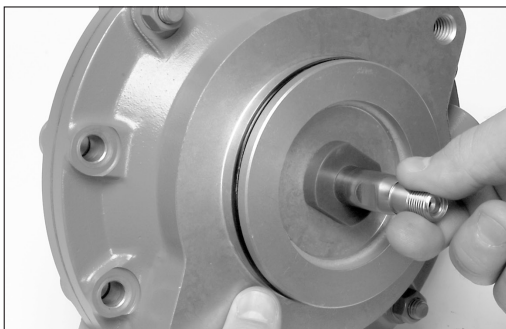
Figure 34 - Checking stem for free movement
