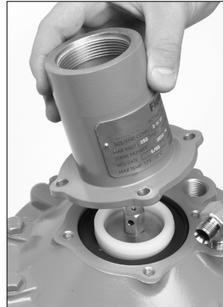
Figure 19 - Removing the spring case
