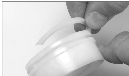
Figure 37 - Installing piston ring on piston
