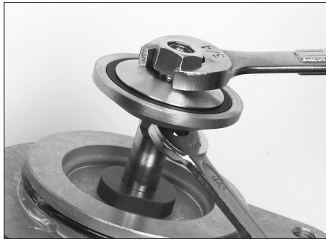
Figure 13 - Hold the stem while tightening the stem nut
