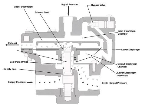
Figure 1 - Cut-away View of BR400 Booster Relay
