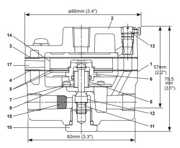
Figure 5 - BR200 Construction and Dimensions
