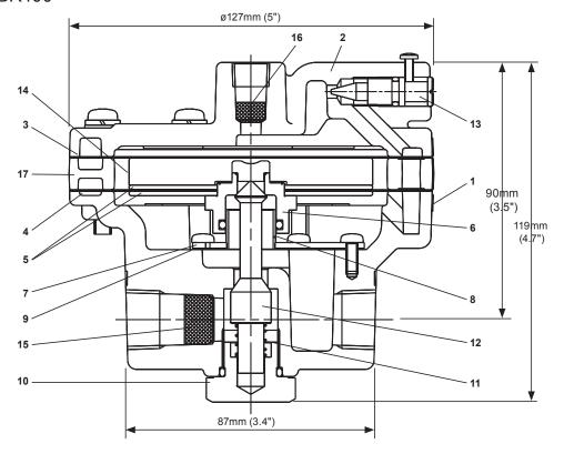
Figure 6 - BR400 Construction and Dimensions
