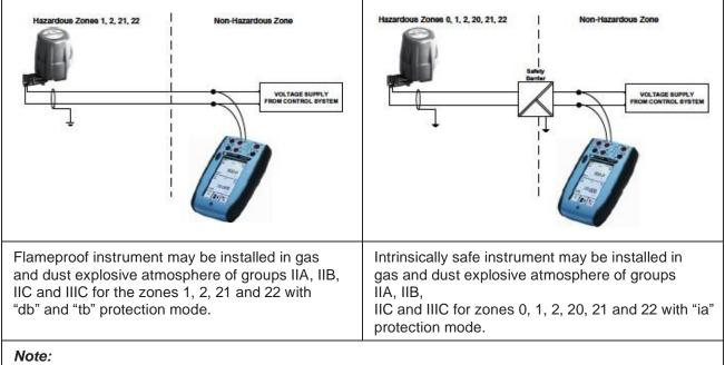
It is under the user responsibility to check the installation against Intrinsic safety rules taking into account entity parameters of all devices in the loop in addition of temporary one like measurement devices.
