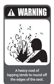
Lap, using a "figure 8" motion in all directions while holding the lap loosely fingers, allowing the weight of the lap to rest on the seat surface. Control the motion of the lap to prevent either the inside or outside edge of the lap from touching the nozzle seat surface. If either edge touches the seat surface the seat can become scratched and rounded.
