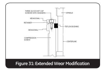
**NOTE:** If the spindle is nickel steel, the existing spindle can be reworked to an extended wear design.
