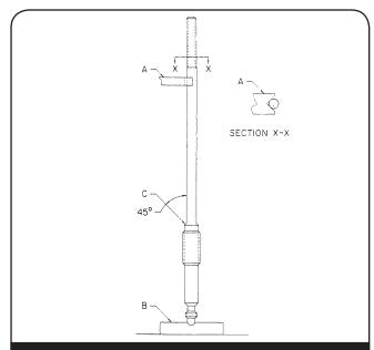
Figure 19: Spindle Runout Determination
