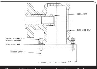
Figure 28: Nozzle Removal and Installation
