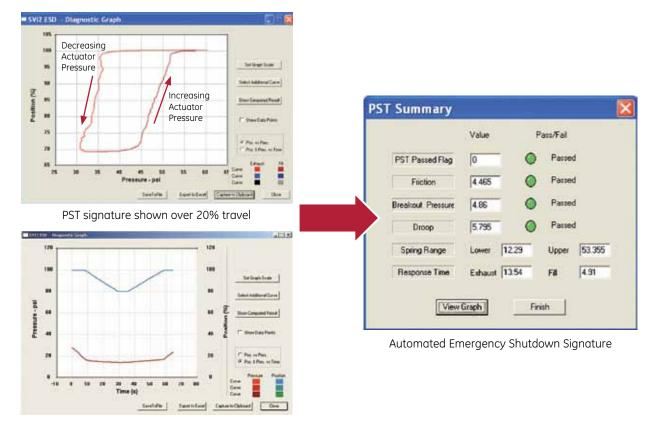
Plotting travel and actuator pressure vs time
