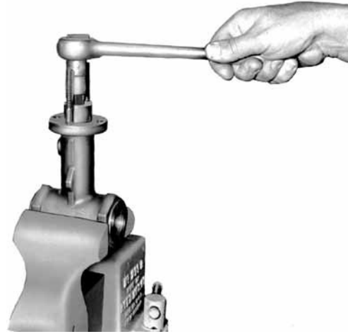
Figure 19 - Tightening the seat-ring retainer (4)
