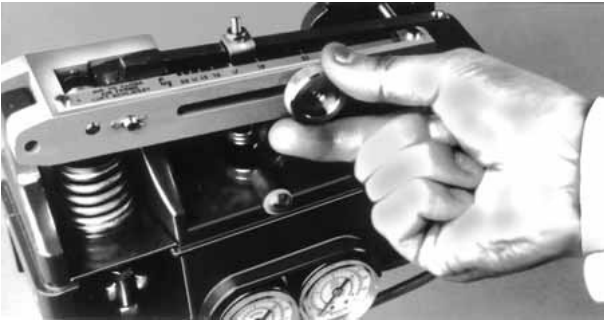
Figure 4 - Adjusting the C v of VariPak 28002 valve for each plug/seat ring combination
