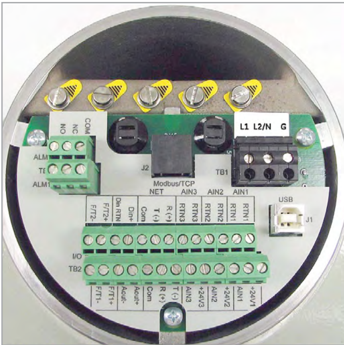
Figure 17: Terminal board with imprinted text (three 4–20mA input option shown)
