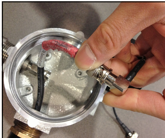
Figure 11: Connecting BNC Plug to Cable
