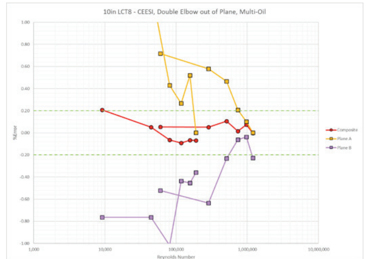
Figure 7. Performance Comparison of the 10-inch LCT8 Against Separated Four-Path Planes
