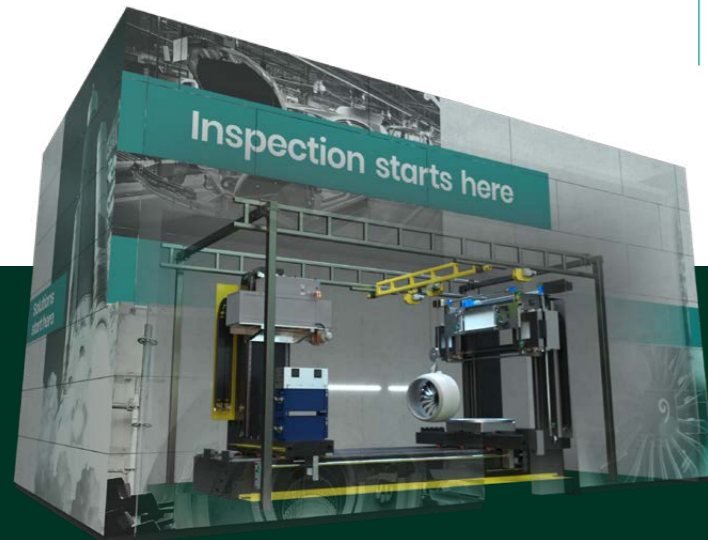
An integrated crane makes loading and unloading of parts that weigh up to 1000 kg simple
