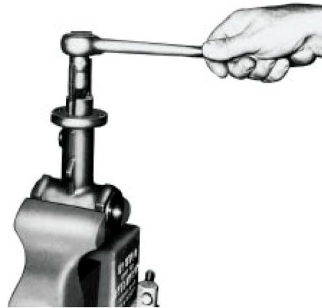
Figure 4 - Tightening the seat ring retainer (4)
