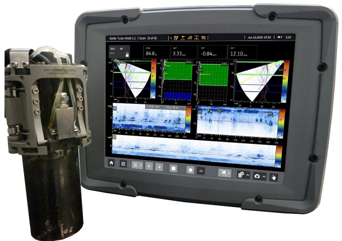
A, C and sector scans show weld indications
