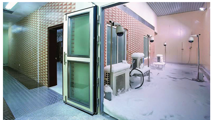
Enthalpy laboratory, extreme temperature simulation, frost can be seen on the ground.
