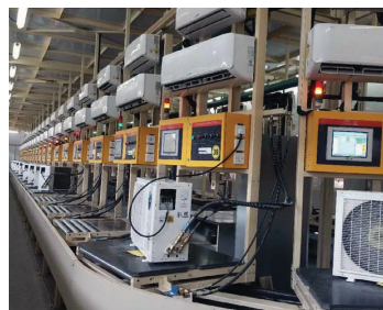
Home air conditioning production line, sensor used for compressor pressure calibration.
