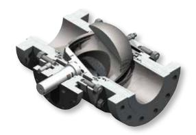
The patented rotary control T-Ball features a non-clogging quarter-turn design that provides quick and low impact automation. Its high capacity and rangeability combined with multi-stage noise attenuating trims makes it ideal for demanding anti-surge applications.
