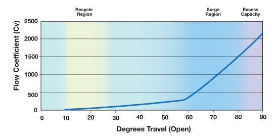
Many cage style valves achieve fast operating speeds by sacrificing the dynamic performance of the valve at low flow conditions. The equal percentage characteristic of a Becker T-Ball offers uncompromising control at both start-up (low flow/high) and surge.
