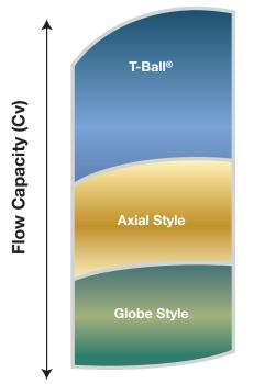
A single Becker T-Ball exhibits the same capacity as two axial or three globe valves.
