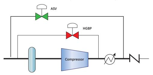
Hot Gas Bypass (HGBP) Valves are employed to provide additional protection against surge. During normal operation, the valve remains closed until a safety critical trip is detected requiring a compressor emergency shutdown. The HGBP valve then springs to open, depressurizing the system as quick as possible by displacing the hot discharge gas into the suction side further preventing compressor surge.
