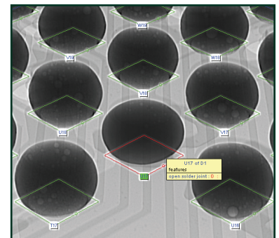
Live CAD overlay and inspection results in the X-ray live image - at any time and at any viewing angle
