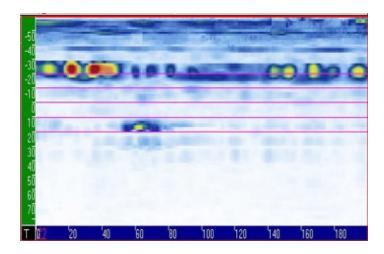
C-scan of weld displaying indications as high reflection signals (red and yellow amplitudes). The weld geometry is displayed in the C-Scan for localization. Cursors are available after the scan for determining the position of indications with respect to the weld geometry.
