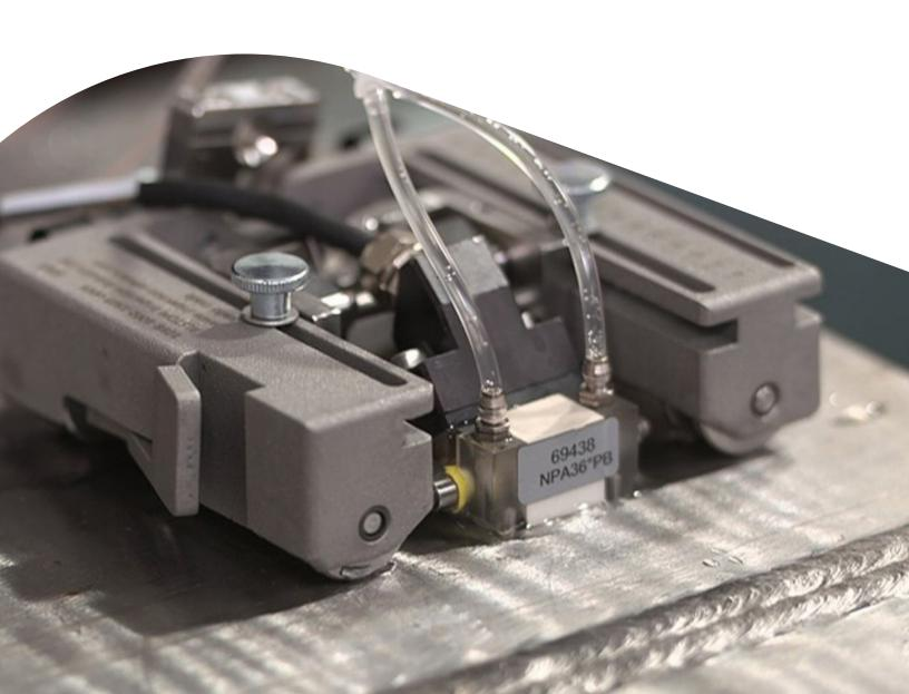
Weld inspections are crucial during the manufacturing process, as well as on a regular basis to ensure weld integrity. Inspections with conventional ultrasonic angle beam probes are time consuming and provide limited documentation. Probability of detection is reduced due to the limited amount of angles used, which could result in missed indications. Waygate Technologies now offers the PALM Flat Scanner to perform more accurate and efficient weld inspections.
