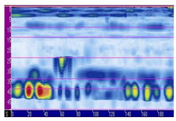
B-scan of weld displaying the depths of indications. The double V weld geometry of a 25 mm thick part is shown. Indications are detected between 1st and 2nd skip in the upper part of the weld at a depth of about 10 mm.
