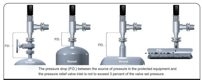
Figure 7: Pressure Drop on the Inlet Piping
