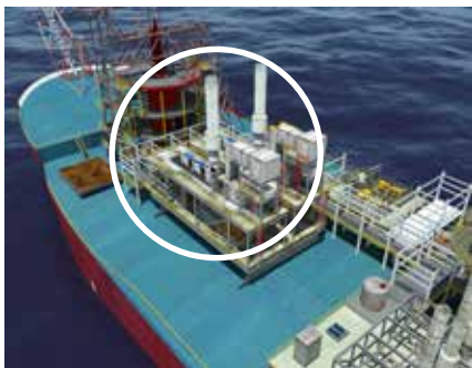
High - Pressure Gas - Injection Compressors
