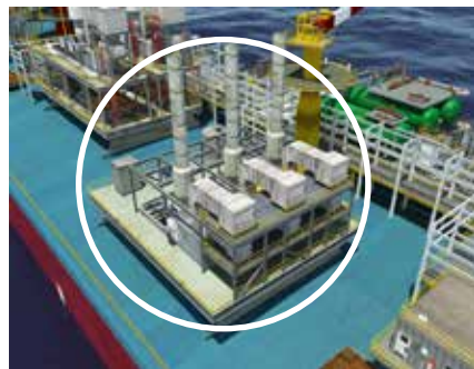
Intermediate - Pressure Gas - Lift Compressors
